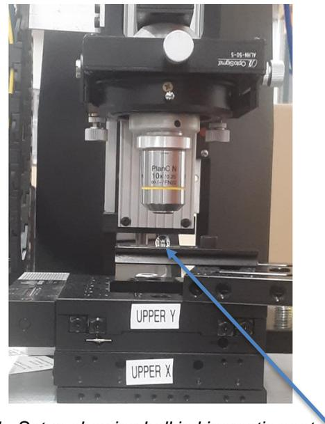
Fig. 1b. Setup showing ball in kinematic seat
