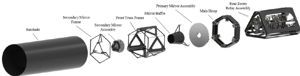
Figure 1. Telescope major subassemblies
