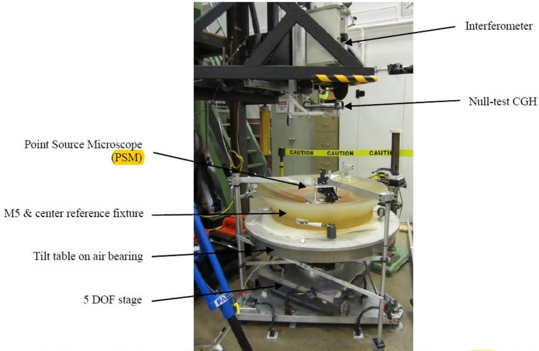
Figure 3. Center reference fixture alignment with the optical axis of M5 using null CGH test and PSM on a rotary air bearing.
