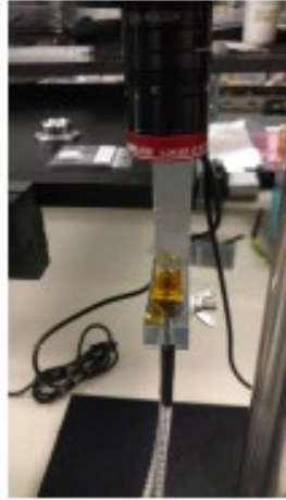
(a) Microscope setup to image the fiberhead during gluing.
