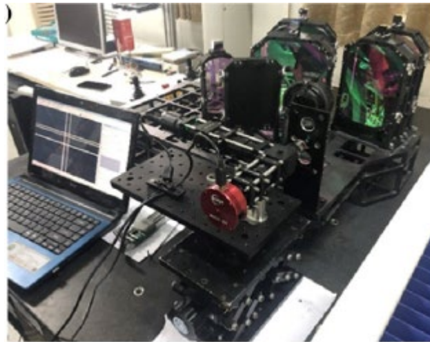
Fig. 19 Adjustment of the spatial position of each optical subassembly by the PSM on the CMM.
