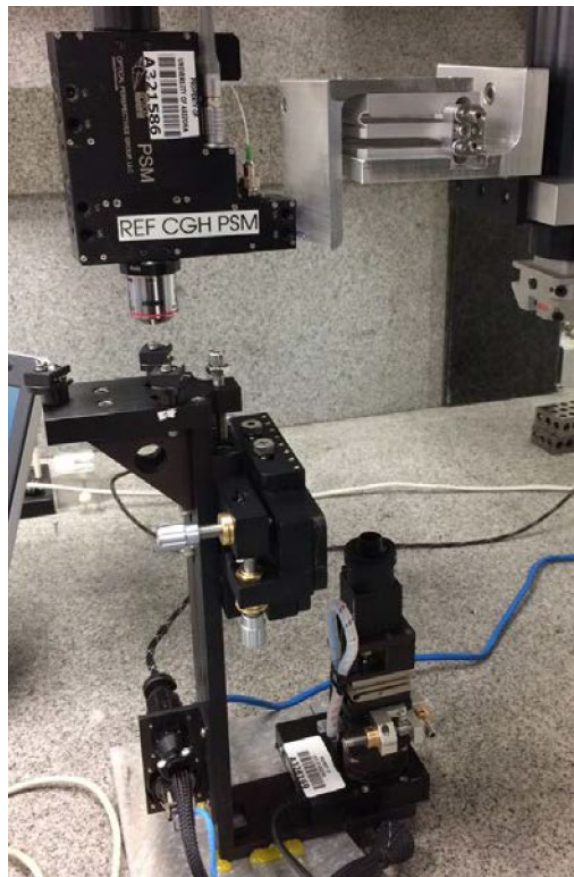
Figure 10. Close up of camera subassembly during calibration. PSM is focused on an SMR.
