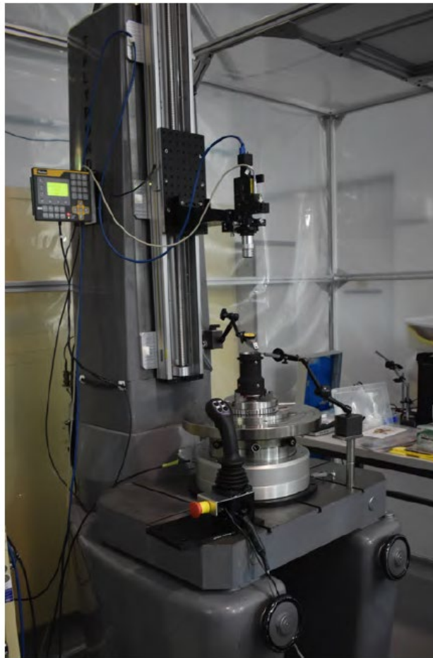
Figure 6. Lens alignment station at Mt. Stromlo Observatory, used to align lenses within barrels with a PSM
