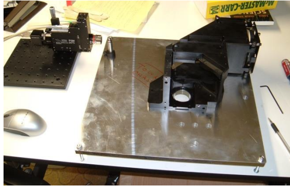
Fig. 11 The PSM focused on the center of a steel ball sitting on the post located in the bored hole in the aluminum alignment plate.
