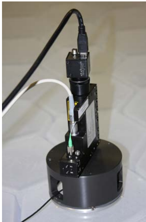
Figure 3.1- MFT picture measuring the surface topography of one of GMT's (8.4 m in diameter) mirrors
