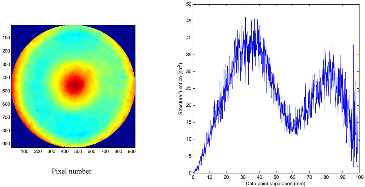
Fig. 4 Contour map (a) of the data used to calculate the structure function (b) using  $10^5$  random data points. The interferogram was 925 pixels square while the aperture was 100 mm in diameter.
