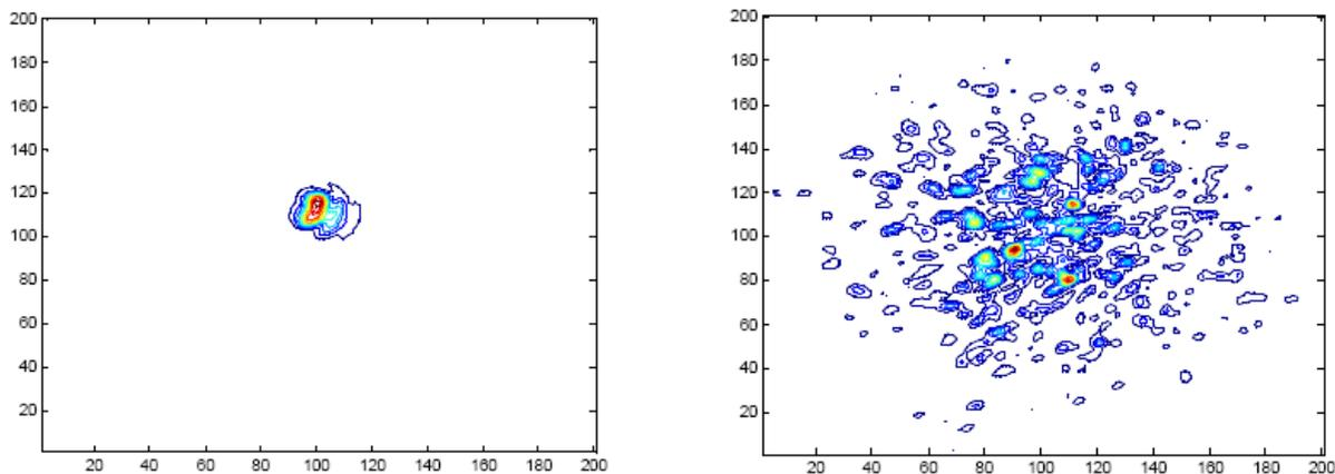
Fig. 1 Image of the first system tested in autocollimation with a FWHM of about  $3 \times 5 \mu\text{m}$  (left). Image of the second identical system tested with a FWHM of about  $20 \mu\text{m}$  (right). The units are detector pixels and the most intense pixels are just under saturation in both cases although the exposure in the right hand image is about 50 times longer than in the left.
