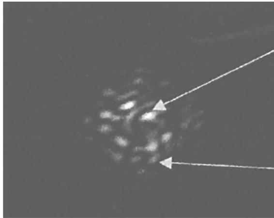
Fig. 2 Image produced by a collimator with point source illumination in autocollimation with brightest pixels at or slightly above saturation
