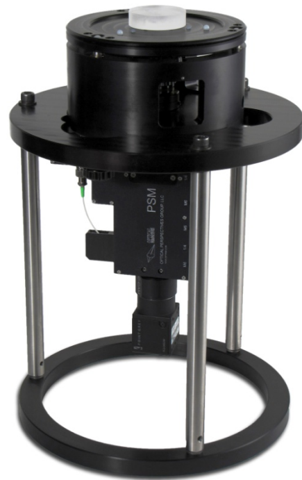
Fig. 6 Photograph of the MFT in its inverted roughness configuration with a small sample on top
